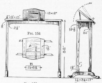
Fig. 152 Fig. 153 Fig. 152, 153 and 154.—Elevations and Details of a Reading Table.
