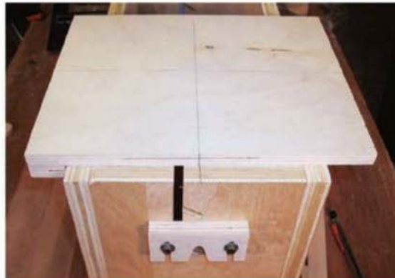
The router slide fits over the top of the jig and is guided by a pair of fixed and spring-loaded fences.
