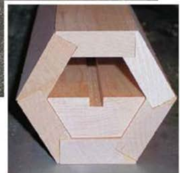
The rolling pin's core consists of two half hexagons with a groove milled along their lengths to house a threaded rod (above). These cores must fit the sleeve interiors snugly (right).
