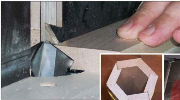
A bird's-mouth bit in the router table (left) forms the necessary cutouts to join six sleeve segments into hexagonal blanks. Glue them together using rubber bands as clamps (first inset). Crosscut them to rough length after the glue dries (second inset).
