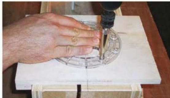
Use the baseplate of your router as a template for positioning it on the slide plate and for drilling mounting screw pilot holes. Bore a through hole in the center for your router bit.
