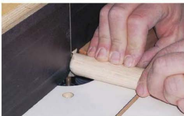
The author milled handles for the rolling pin by routing four 1/2" roundovers into a piece of 1" x 1" stock (top). He then rounded over the ends of each handle with the same bit (bottom).
