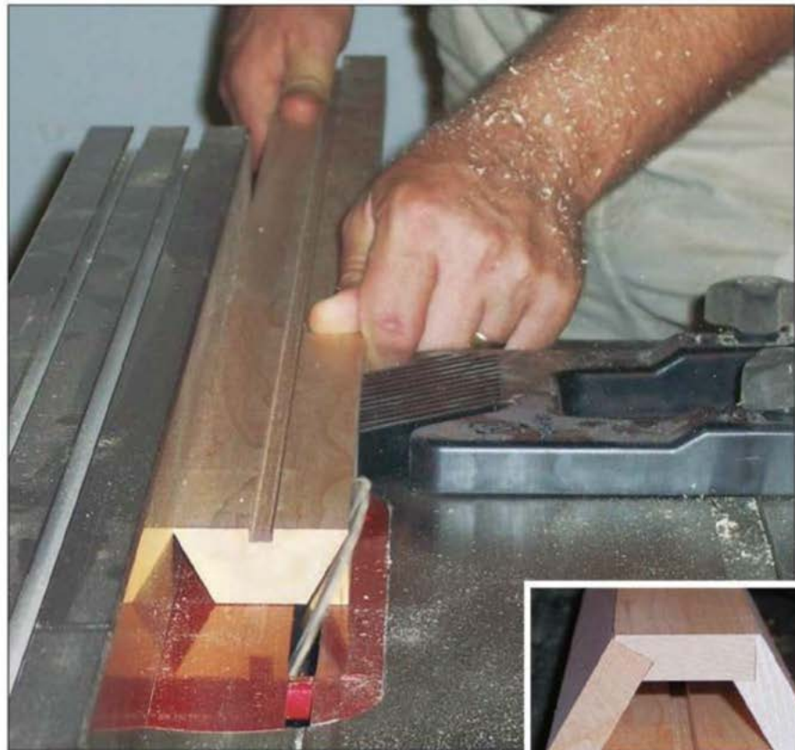
The rolling pin's core consists of two half hexagons with a groove milled along their lengths to house a threaded rod (above). These cores must fit the sleeve interiors snugly (right).
