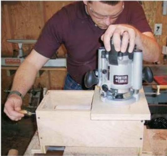
Shaping each sleeve into a cylinder is a process of slowly moving the router slide across the jig while simultaneously turning the sleeve. It's a two-crank operation.
