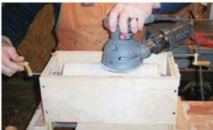
Forming the grooved sleeves involves plunge-routing each groove one at a time, then turning the indexing crank a specific number of turns to set up for the next groove (top and center). You can power-sand all three of the sleeves easily without removing them from the jig (bottom).
