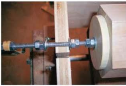
Jamb nuts and washers lock the handle and sleeve blanks on the threaded rod for milling. The whole assembly seats in the jig slots.
