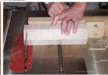
A bird's-mouth bit in the router table (left) forms the necessary cutouts to join six sleeve segments into hexagonal blanks. Glue them together using rubber bands as clamps (first inset). Crosscut them to rough length after the glue dries (second inset).
