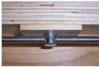
A cross dowel nut, engaged in a hole in the cross dowel bracket, moves the router slide back and forth on the indexing rod.
